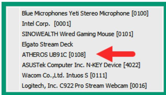
Figure 7.36 – Selecting the wireless network adapter
